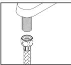
(4) When using stainless steel braided faucet supply hose; this faucet requires one end of the supply hose to have a 1/2" female IPS connection. The other end of this supply hose must match the thread on the water supply valve under your sink. Once you've identified the required size, carefully follow the manufacturer's installation instructions for each hose
