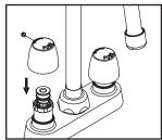
(8) Once the satisfactory timing has been adjusted, install the handle by tightening Allen
